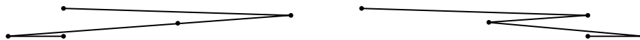
Figure 1. A carpenter's ruler with segments of length 1, 3, 2 and 4 folded so that it fits into a case of length 5 (left). Its folding vector is (-1, 1, 1, -1) . Another folding into a case of same length (right). Its folding vector is (1, -1, 1, -1) .
